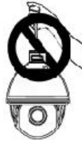
2. Don't pick up the cable by hand, it may cause connection problem with cable.
