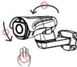
4. To make sure the product work properly, don't rotate pan and tilt parts by force, to avoid rotating parts displaced or motor damaged.
